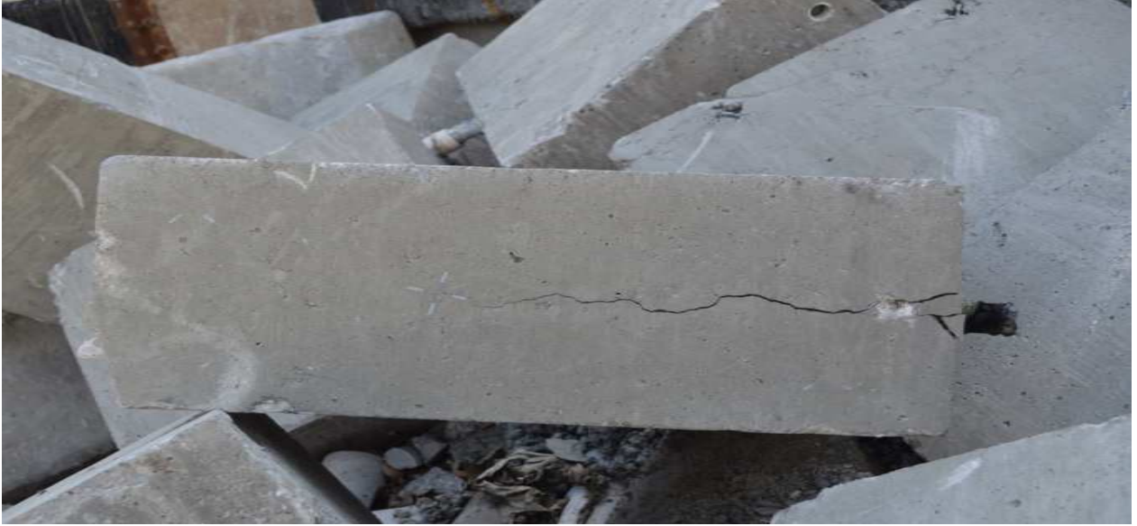
Figure 1 Original Cracked Concrete Block Image (DSLR Camera)
